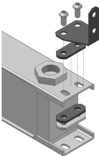
These brackets assist in the mounting and protection of the oil cooler; however, mounting an oil cooler with these brackets is no guarantee of protection or substitute for common sense.
