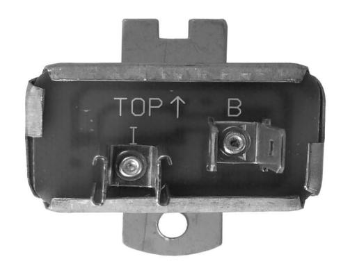
Smiths Classic bimetal gauges operate on a stabilised 10 volt supply. A healthy car battery will supply somewhere in the region of 13.5 volts. A voltage stabiliser must be fitted to the guage supply line. There are many variants of the SMiths voltage stabiliser but the connection should remain the same.
